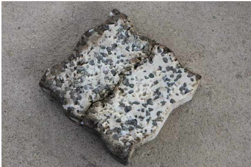
Weaker ecobricks made from densified plastic. The gravel is added for traction.
