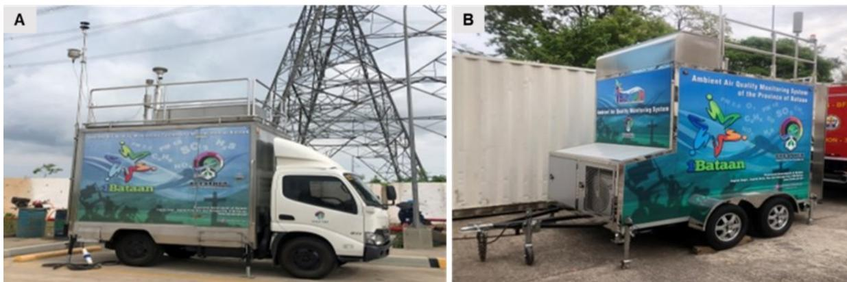
Air quality monitoring system (AQMS) of the Province of Bataan consisting of (A) mobile and (B) trailer-type units.
