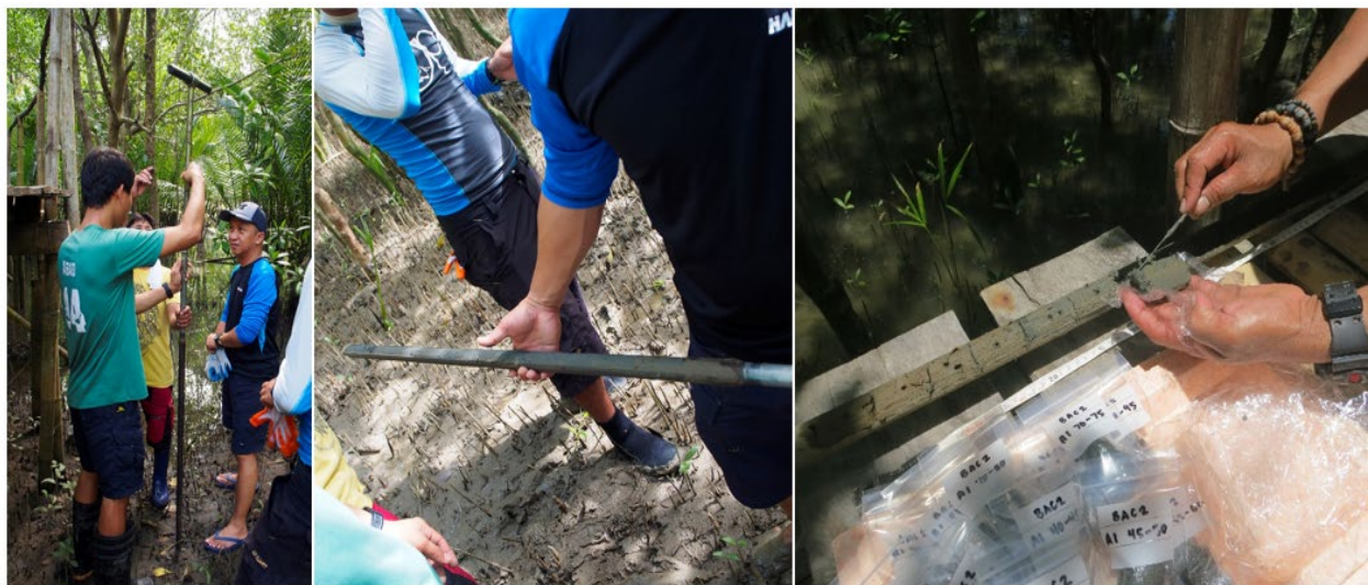
Figure 15: Sediment collection using auger in the field
